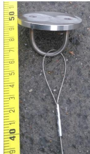
The cable, in combination with the well cap and eyebolt, is preassembled at the right length
