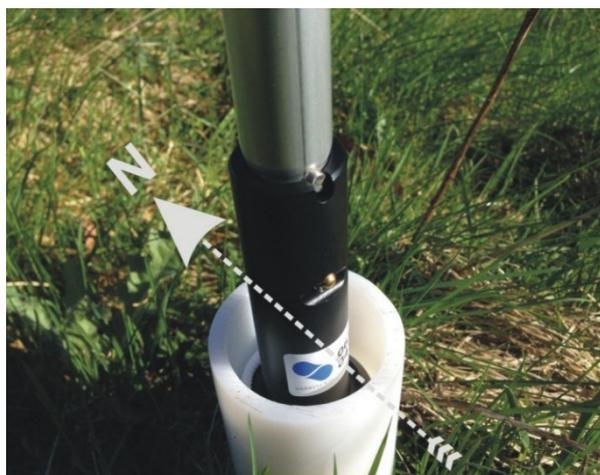
*Left: schematic of Fluxsampler with three peripheral sorbent sections and centre core of tracer salt; right: picture of Fluxsampler in groundwater filter casing.*
