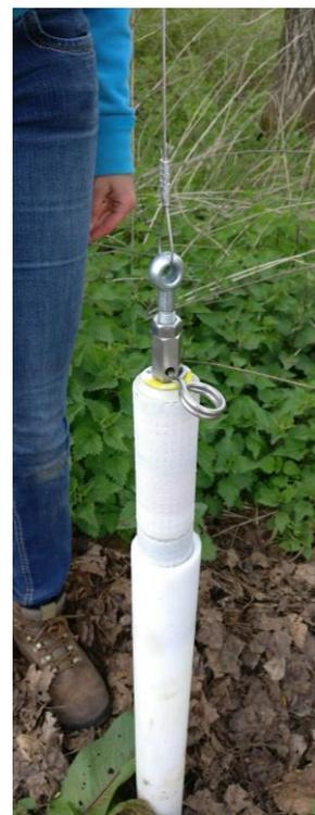
\*Locking pin is used to avoid sudden drop in the well
