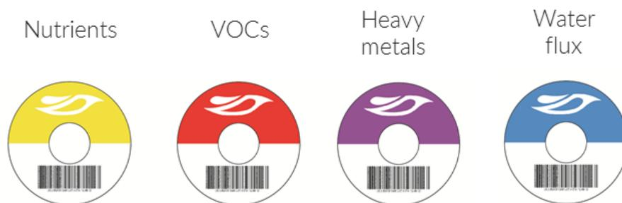
Each iFLUX cartridge is 15 cm long and has a outer diameter of 4.9 cm. Different cartridges can be combined modularly as an iFLUX sampler, depending on the different types of pollutants and the different desired depths. The material used has been extensively tested and meets all the requirements for correct soil remediation. The used tracers are methanol, ethanol, 2-propanol, tert. butanol and 2,4-dimethyl-3-pentanol and do not involve any environmental risk.
